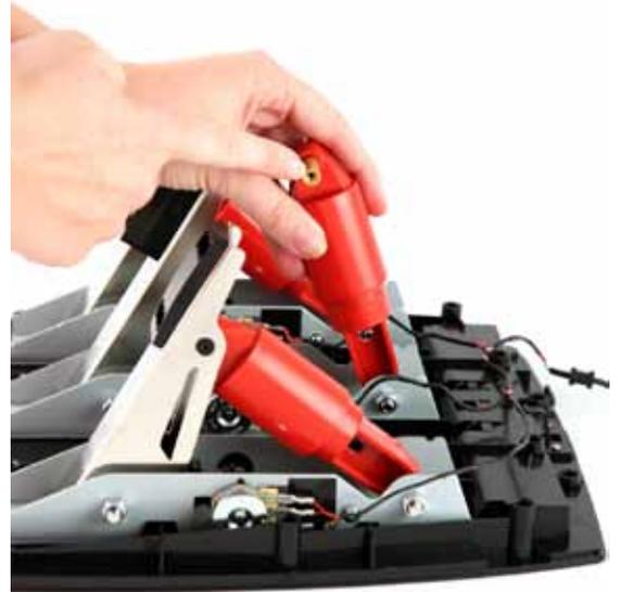
6. Remove upper half of plunger to reveal original spring.
