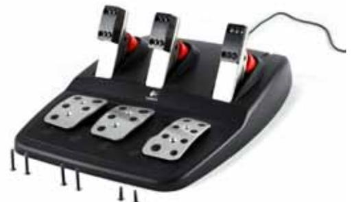
3. Underneath the pedal set, locate and remove 14 silver screws.
