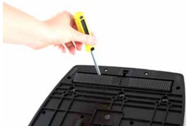
4. Separate base plate and cover, be very careful not to overstretch the fine wires located inside.
